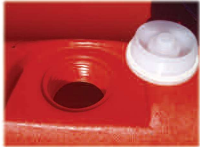
New tamper resistant, corner offset drain plug with coarse buttress thread — screws in or out in only 2 1/2 turns.
